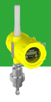
The Accutech™ TM10 wireless turbine meter field unit measures the volumetric flow rate of liquids or gases by detecting the frequency of pulses generated with a standard turbine meter (not included) and applying a user-configured proportional "K" factor. A 22-point correction curve is used as a final offset or for custom calibration of turbine meter as required. There are two principal outputs providing flow rate and totalised flow measurements.
