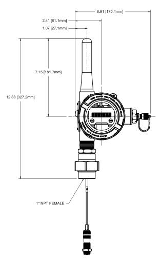
2.4GHz INTEGRAL ANTENNA AND CABLED ANTENNA OPTIONS
